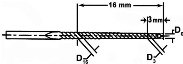
INSTRUMENT WITH TAPER UP TO 4%
